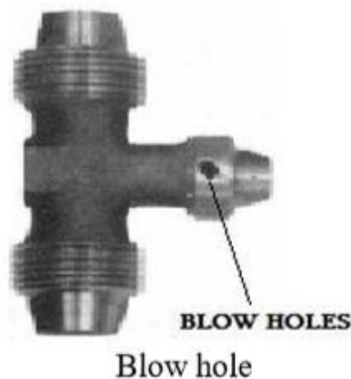
Figure-1: Blow hole defect
